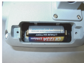
C Replace battery P/N 2239138
